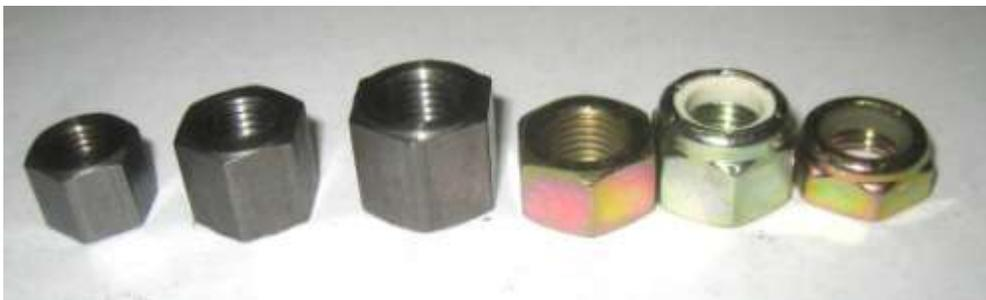
The photo shows a  $7/16^{th}$ ,  $1/2$  inch and a  $9/16^{th}$  in 1.5 length. The 3 on the right are normal, nylock normal and half nylock.
